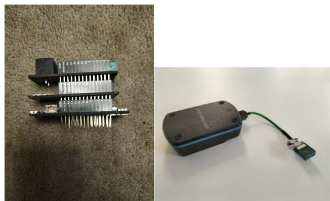
Figure 2: Analysed wireless systems to measure temperature from thermocouples and transmit temperature data
