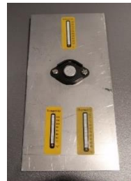
Dummy for T measurement at datalogger position
