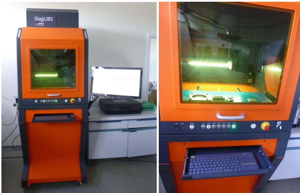
Figure 1: LIBS device in the laboratory (left) and measuring room with cover (laser protection glass) and controls (right)
